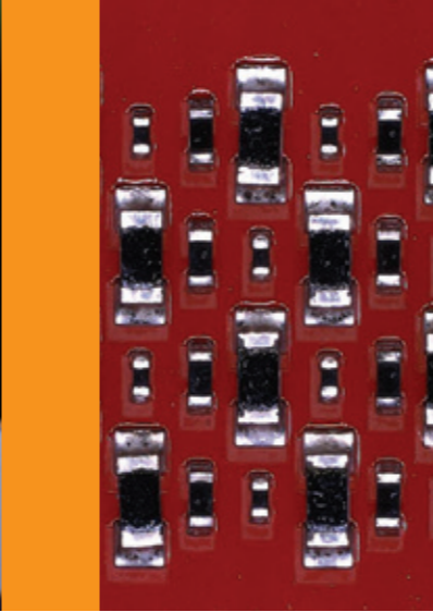
Resistors sized 01005 to 0402
