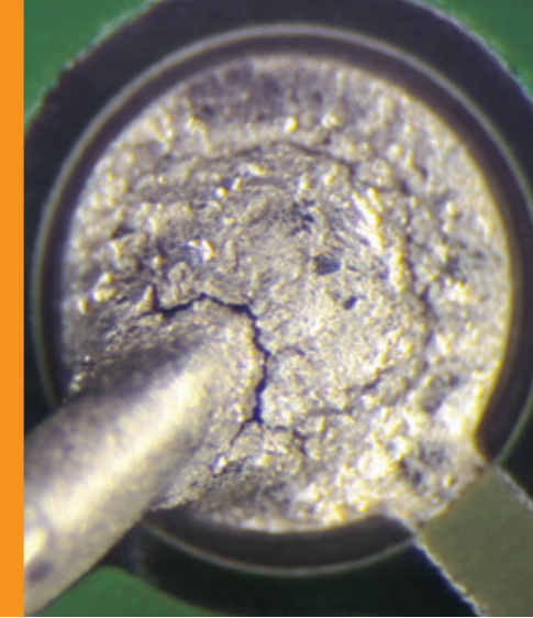
THT-solder joint with fatigue crack
